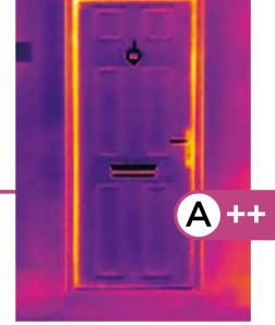
**APEER A++ DOOR** The door is showing in cool colours meaning heat is NOT escaping through the door.
